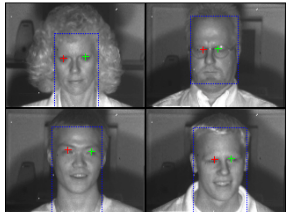
Figure 11: Examples of the system's performance in frontal faces. The images belong to the lower near-IR stream and are superimposed by the skin box and the crosses indicating the locations of the eyes.
