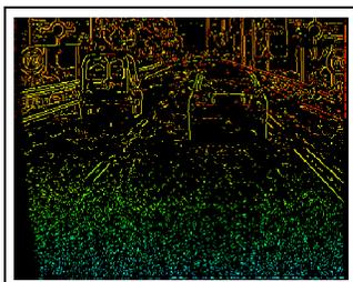
Fig. 7. Disparity map computed by the proposed method.
