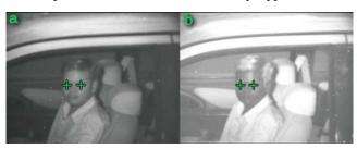
Fig. 32. Example of our system detecting the driver of a car in an outdoor environment. (a) Low near-IR image with the eye positions overlaid in green. (b) High near-IR image with the eye positions overlaid in green.
