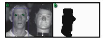
Fig. 6. (a) Example of successful discrimination between a real and an artificial human head, (b) The binary output of the skin detection process.
