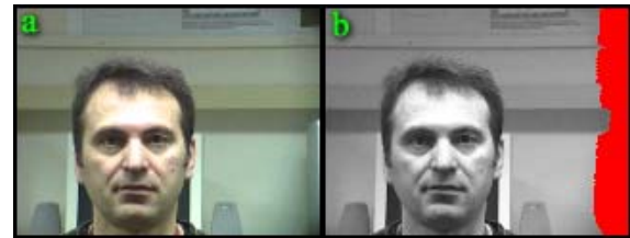
Figure 10: An example of the integral projection in the visible band. (a) The visible band image. (b) The gray scale version of the visible band image with its integral projection overlaid in red. The dark stripe in the background creates a significant valley that would make eye detection very hard.
