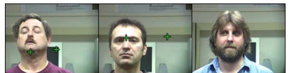
Figure 30: Example output of the Identix FaceIt ® face detector performing poorly on frontal faces. The location of the eyes reported by the detector is marked with green crosses.
