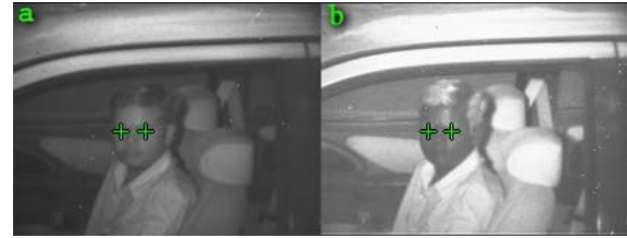
Figure 32: Example of our system detecting the driver of a car in an outdoor environment (a) Low near-IR image with the eye positions overlaid in green, (b) High near-IR image with the eye positions overlaid in green.
