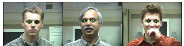
Figure 29: Example output of the Identix FaceIt ® face detector performing well on frontal faces. The locations of the eyes reported by the detector are marked with green crosses.
