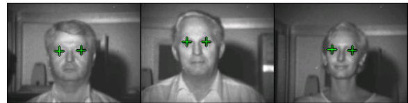
Figure 26: Examples of the proposed system's performance using frontal faces. The superimposed crosses indicate the locations of the eyes.
