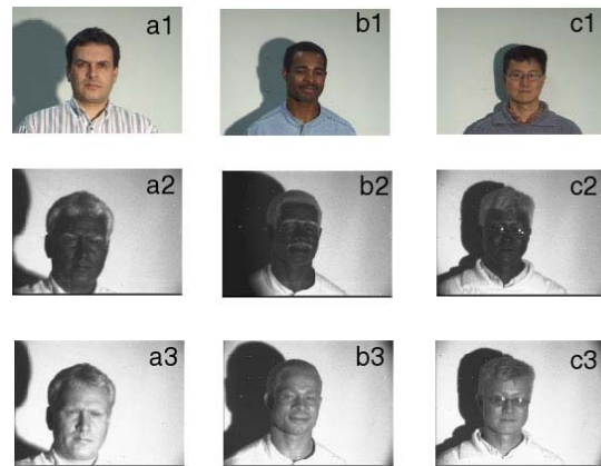
Figure 21: Three of the subjects used in our data set as they appear in the visible, upper near-IR, and lower near-IR bands. The subjects are representative of the Caucasian, African, and Asian groups.
