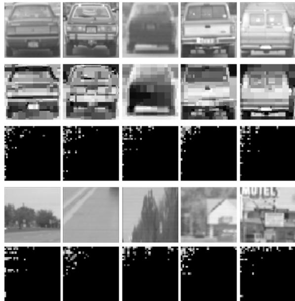
Figure 1: 1st row: vehicle sub-images used for training; 2nd row: reconstructed sub-images using the top 50 coefficients; 3rd row: illustration of the top 50 quantized coefficients; 4th and 5th rows: similar results for some non-vehicle sub-images.
