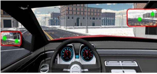
Figure 10: The user's eye gaze tracked by the FOVE virtual reality headset. Our system detects whether the user has looked at the rear-view driving mirrors (red). His eye gaze (green) is recorded from the FOVE virtual reality headset for analysis.
