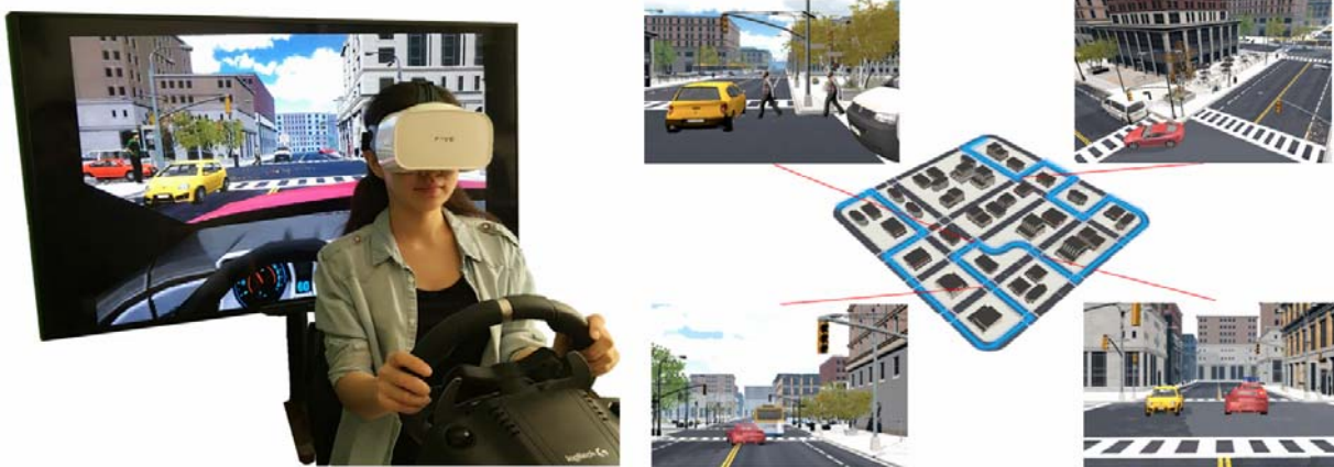
Figure 1: A user is practicing with a personalized training program synthesized by our approach to improving her driving habits via virtual reality. Left: our system is constructed using a Logitech driving controller and a FOVE eye-tracking virtual reality headset, via which the user's driving and eye gaze data are collected for analyzing her driving habits. Right: A training program (blue route) is synthesized by our approach for improving the user's driving habits via different traffic events.
