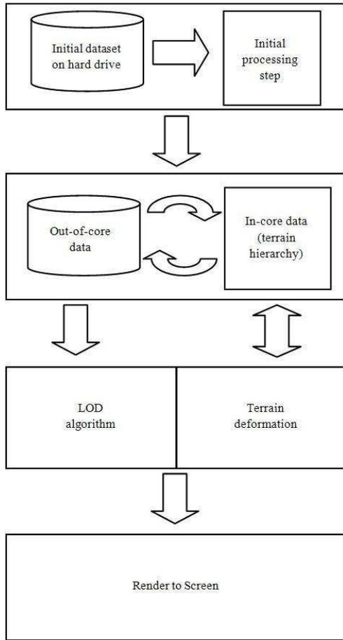
Figure 1: Block diagram demonstrating the flow of the data through the system
