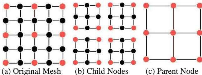
Figure 2: The simplification process to create a quadtree. The original mesh (a) is separated into  $m \times m$  nodes ( $m=5$ ) (b), where each  $2 \times 2$  block creates a parent node (c)
