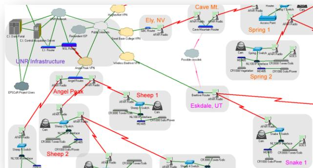
**Figure 4.** The overall communication network that integrates remote data loggers with the SENSOR system for the Nevada Climate Change Project.
