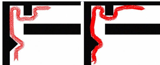
Figure 3. (a) The path taken by the teacher during wall training. (b) The path taken by the robot in the environment after learning the desired behavior.
