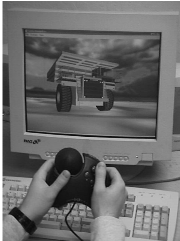
Figure 1: A Person Conducting an Inspection with a SpaceOrb by SpaceTec [6]
