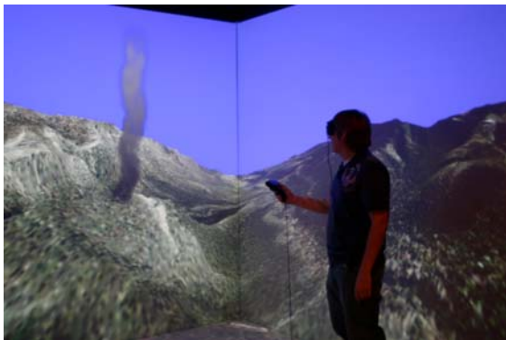
Figure 2: Smoke is rendered using a particle system based node in OpenSceneGraph. A similar method is used to visualize fire.
