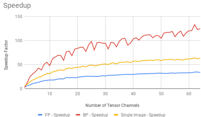
Fig. 4. Speedup of these methods start to slow down between 10-15 tensor channels (360-540 lower level capsules) as these methods increase due to Amdahl's law. Note that back propagation, which only communicates resulting \mathbf{v}_j errors back to the host, a constant k \times d_{l+1} = 160 values, has higher speedup than forward propagation, which requires the movement of a 28 \times 28 sized image from the MNIST dataset. [7].
