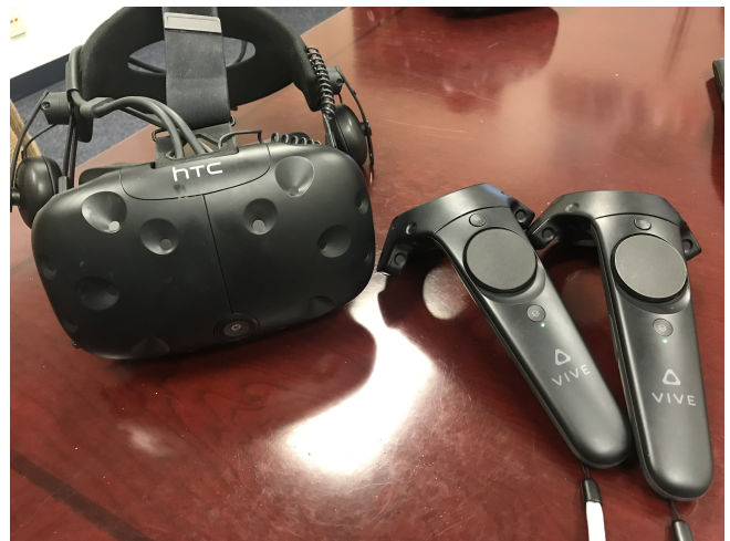
Fig. 1. (Left) HTC Vive Headset. (Right) HTC Vive Controllers with adjustable straps.
