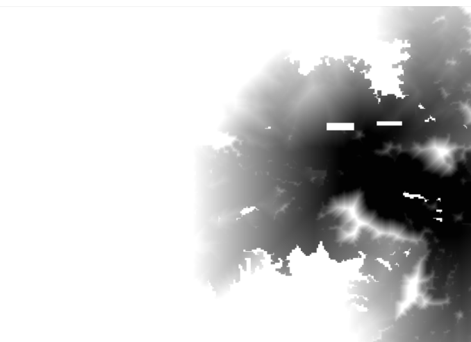
Fig. 5. The burn map generated from a successful run of vFireLib's simulation. float values are passed in and saved into an exr format to preserve the 32bit floating point time of arrival information.
