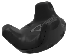
Figure 3. Additional trackers for the HTC Vive that allows for more tracked parts of the body or additional objects. [8]
