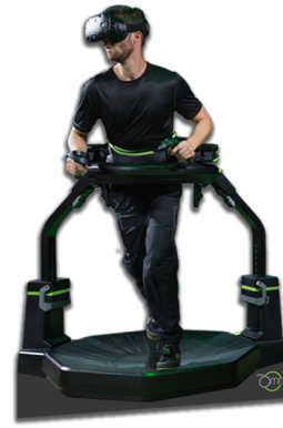
Figure 1. The Virtuix Omni, a passive omni-directional treadmill, allows a user to run/walk in place, and allows the user to steer based off of the direction of their hips [22]
