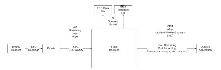
Fig. 4. High level diagram of data being recorded and capture from Emotiv's lab streaming layer in a Flask Backend.
