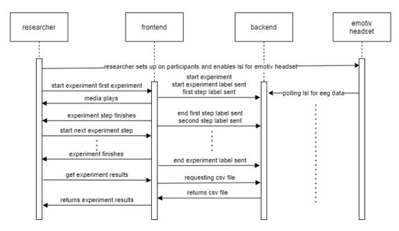
Fig. 2. Sequence diagram of the flow from the researcher starting the experiment and the experiment as a whole.
