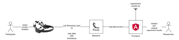
Fig. 1. A diagram showing the whole system regarding the data flow and interactions with the research and participant.
