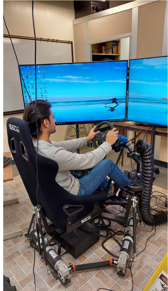
Fig. 1. The truck driving input and output system with a user seated inside.
