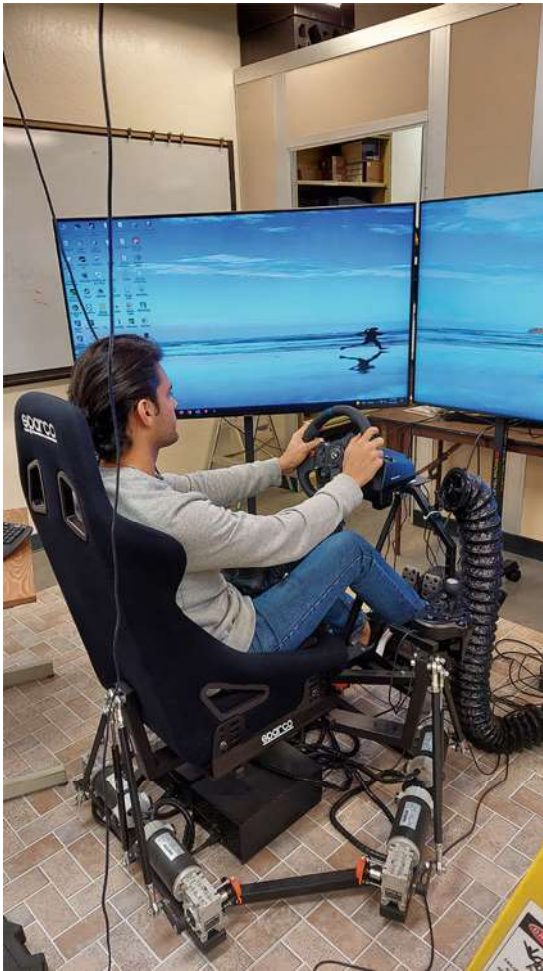
Fig. 44.1 The truck driving input and output system with a user seated inside
