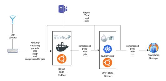
Fig. 1. High level diagram of the proposed pipeline architecture showing the flow of the PCAP from the edge to Pronghorn.
