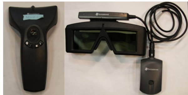
Figure 3: (Left) A 6-DOF wand device. (Right) A 6-DOF tracking device mounted on stereoscopic glasses.
