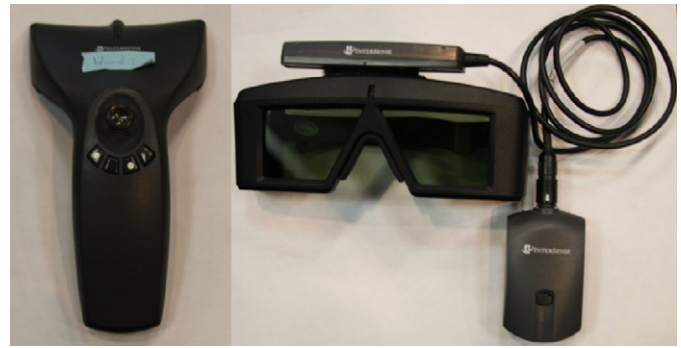
Fig. 3. (Left) A 6-DOF wand device. (Right) A 6-DOF tracking device mounted on stereoscopic glasses.
