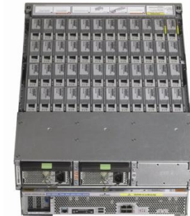
Sun 4600s and 4500s 16 core boxes with 200GB of RAM connected by Infiniband And several 24TB disk arrays
