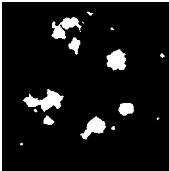
Figure 18: Image 2 after border particle rejection.
