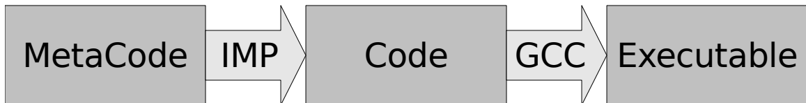
Figure 3.1: Added stage in the IMP compile process
