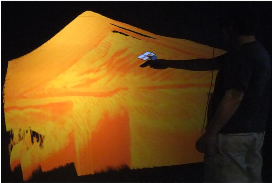
Figure 5.14: Brunton Compass Tool being positioned in the GPR data to take a measurement with snapping enabled.
