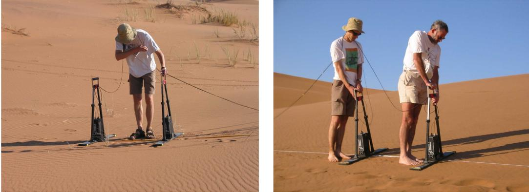
Figure 2.2: Researchers using a GPR unit in the field on a sand dune.
