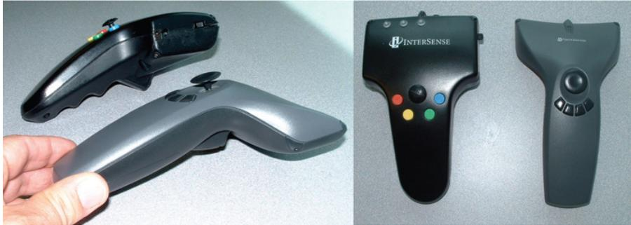
Figure 2.23: Two 6-DOF wand devices [72].
