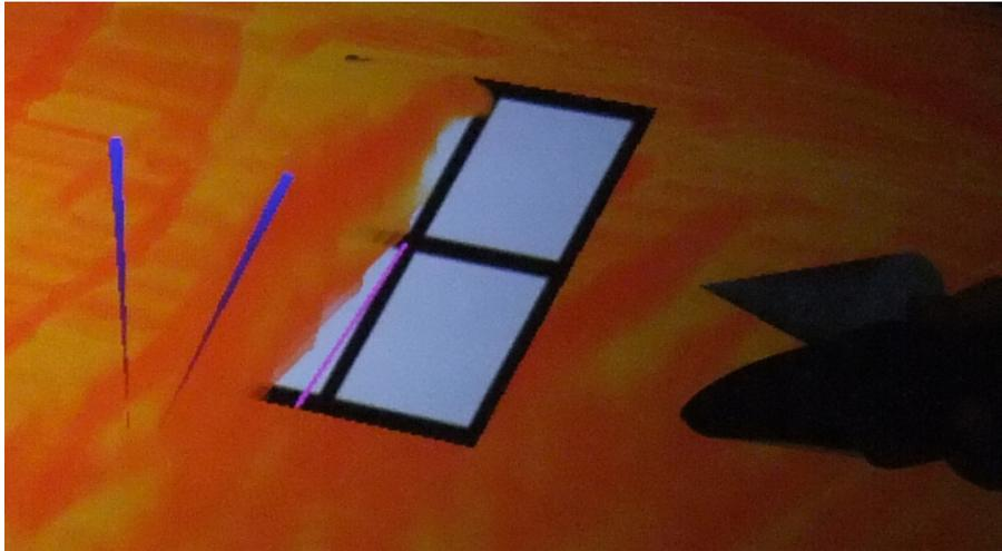
Figure 5.16: Brunton Compass Tool with several saved measurements and steepest gradient visible.
