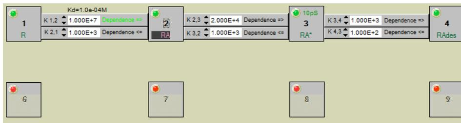
**Figure 2.8:** ChannelLab 2D grid layout of a four state model connected with six rate constants.
