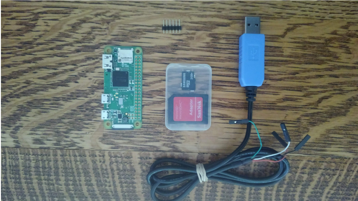
Figure A.1: Required Hardware sans PC
