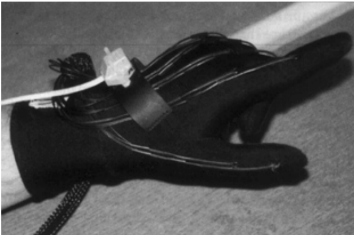
Figure 2.3: The VPL Dataglove used resistive sensors in order to allow a richer interaction than a three dimensional mouse. It allowed the user to use hand gestures that were recognized and translated into proper actions [25].
