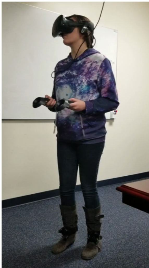
Figure 2.7: This participant has trackers attached to her ankles over her boots which keep track of where her feet are in space. As her feet oscillated, she was propelled forward in the direction she was gazing in the virtual environment.
