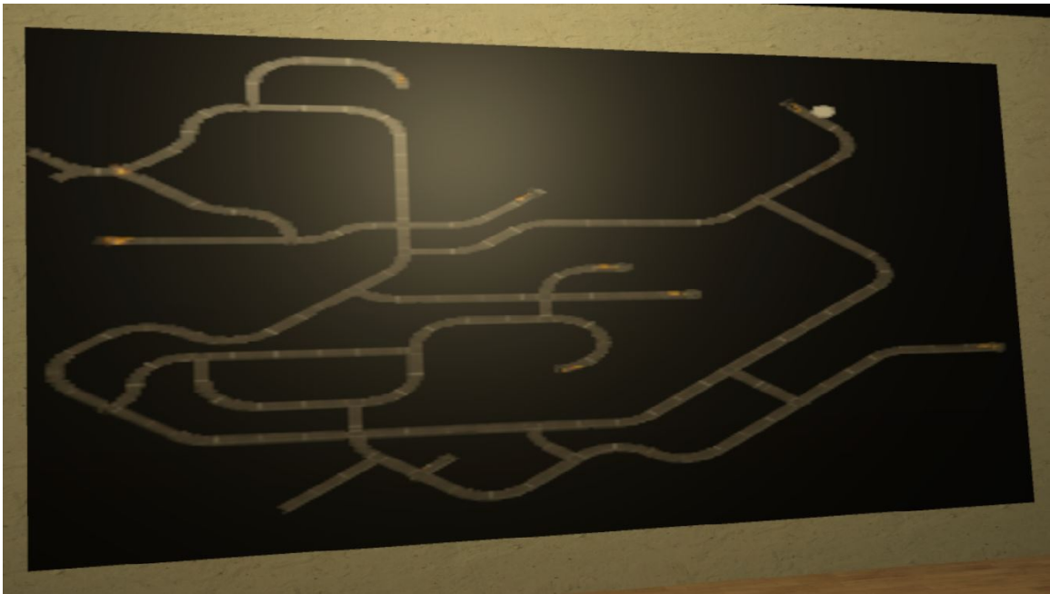
Figure 5.3: The overall map of the mine as seen from the users perspective in the control room. The white disc on the map represents the user inside of the mine. The orange lights represent hazards within the mine, in this case, fires.
