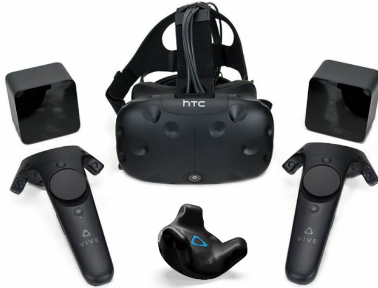
Figure 5.1: The HTC head mounted display along with the two lighthouse trackers, two hand remotes, and a single extra tracker(two of which are used in this experiment) [11].
