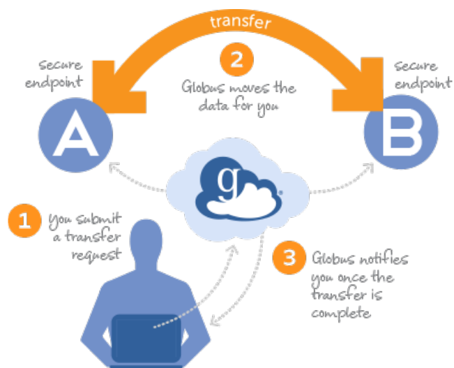
Figure 2.11: A high-level representation of the Globus workflow for researchers [84].
