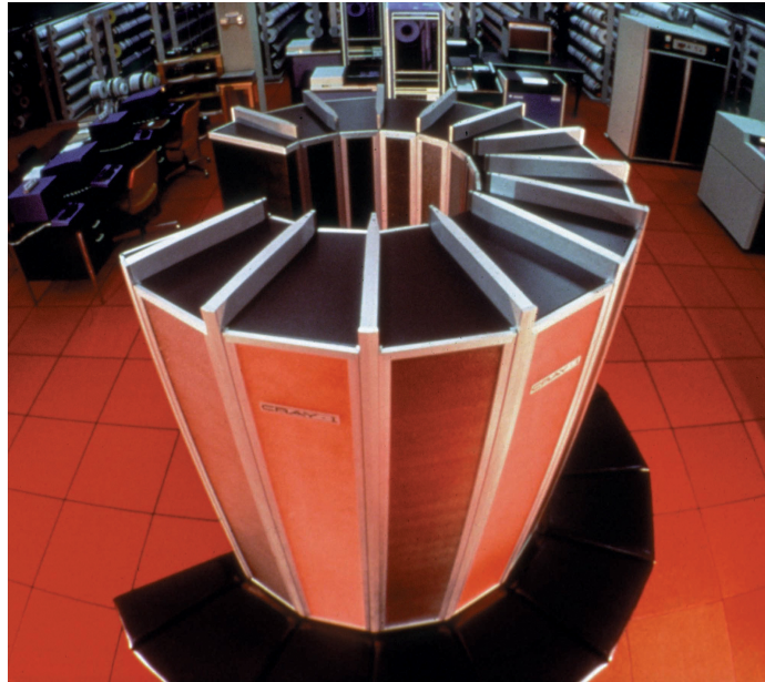
Figure 2.5: The Cray-1, released in 1976, was among the first supercomputers and the first computer to allow parallelization [38].
