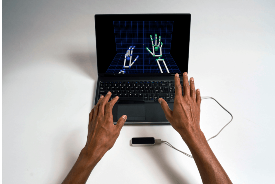
Figure 2.13: A user’s hands being tracked by the LEAP motion device and the resulting skeletal figures provided by the accompanying SDK [37].
