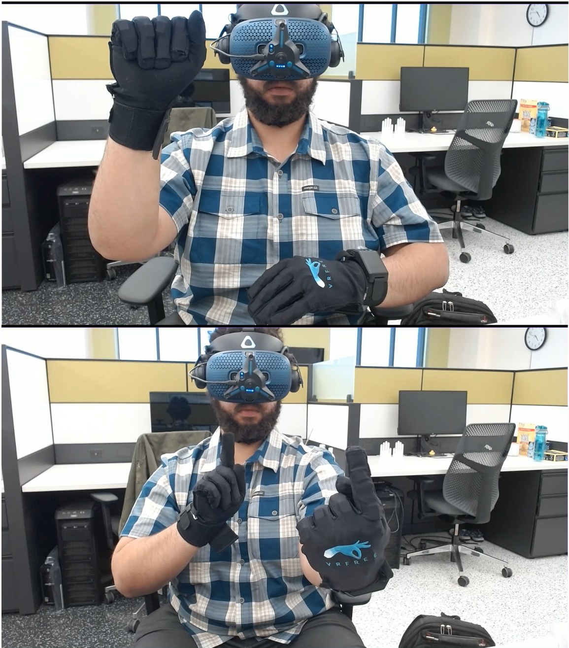
Figure 4.1: A user equipped with the two primary components of the apparatus: the Vive Cosmos VR Headset, and the VRFree Gloves.
