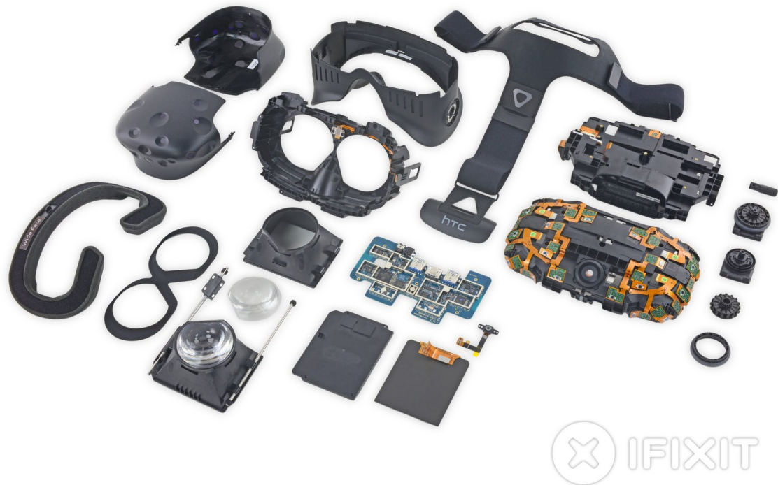
Figure 2.8: The individual components of an HTC Vive headset displayed after a disassembly [17].
