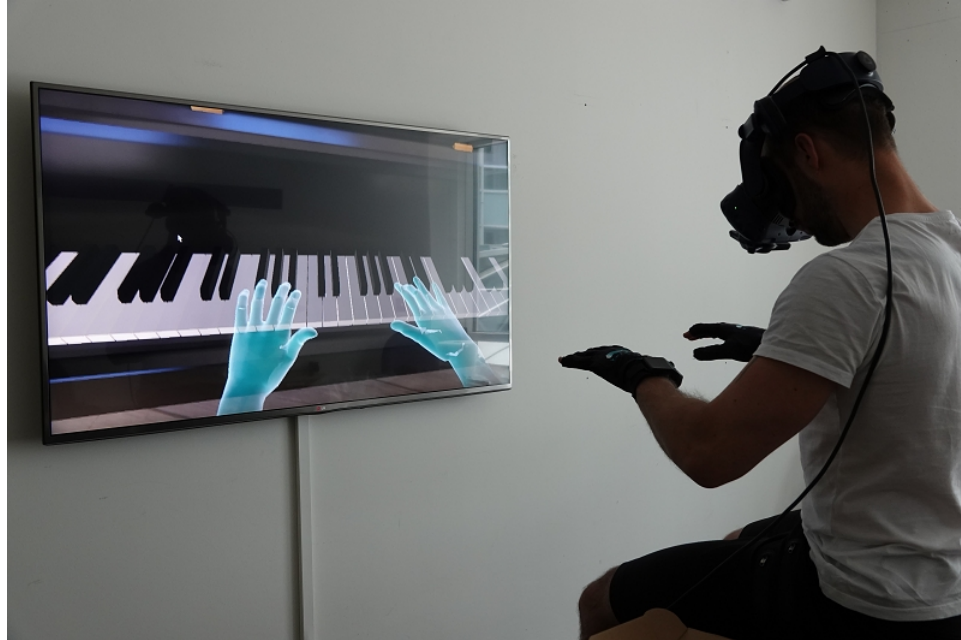
Figure 2.15: An image demonstration of the tracking capabilities of the VRfree glove system. A user plays a virtual piano using the gloves which is one of many possible activities that can be performed in the demo application provided with the glove SDK [25].
