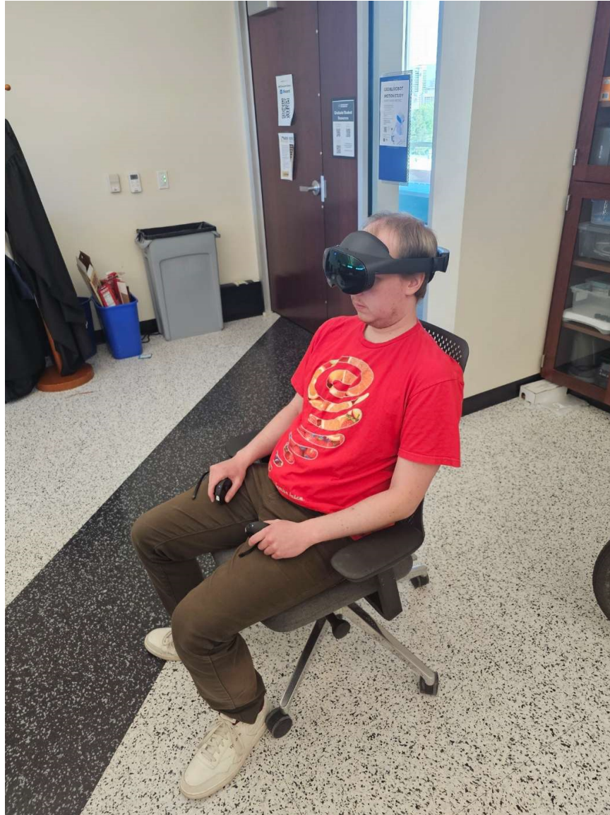
Figure 5.1: The hardware used for this experiment was the Oculus Quest Pro. This headset was chosen due to its adaptability for glasses, as well as the hope that new users would be less worried about being cut off from real life.
