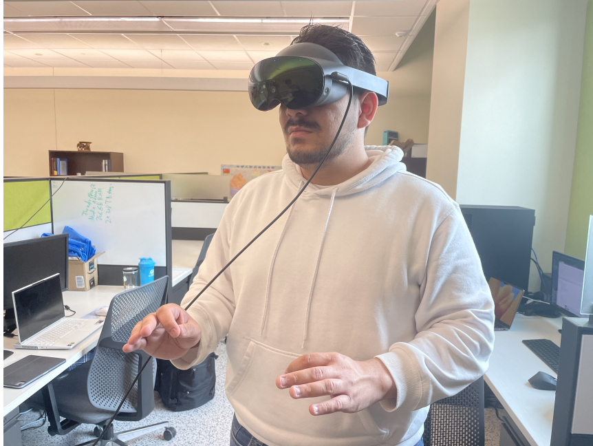
Figure 4.2: The Meta Quest Pro head-mounted display allows for the usage of hand-gesture recognition through auxiliary cameras.
