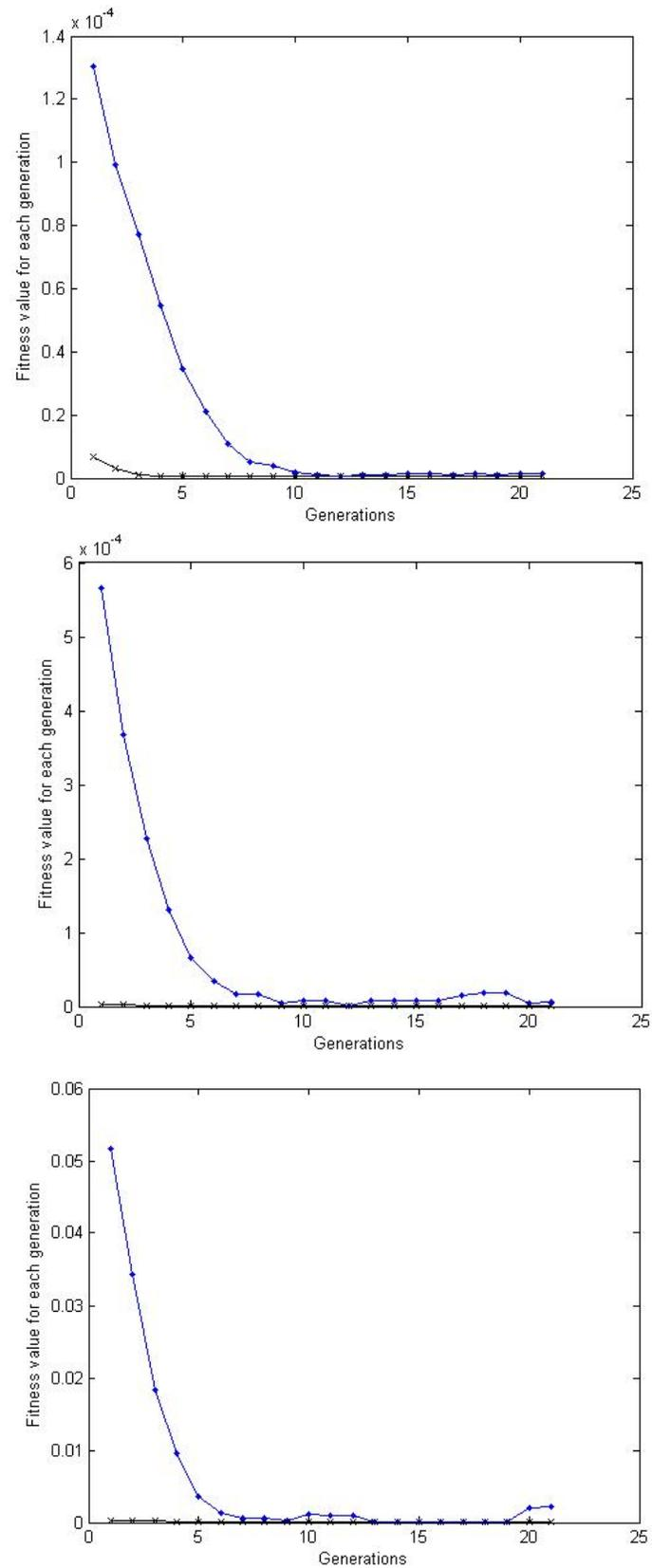
Figure 5.6: In running for 20 generations with a population size of 100, the change in best fitness value and the mean fitness value: (a) for vertex index 10 of the Smiley, (b) for vertex index 10 of the Mannequin, and (c) for vertex index 20 of the Mechanical
