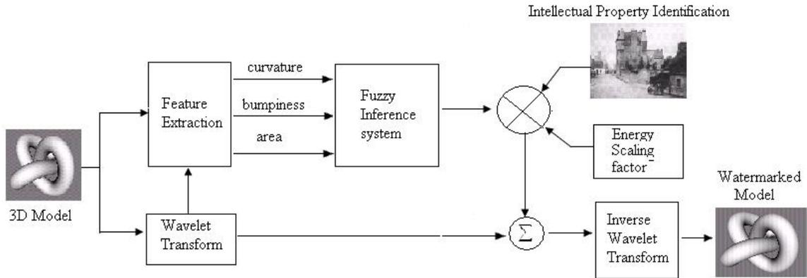
Figure 4.1: Fuzzy Logic Based Approach - Block Diagram for Watermark Embedding identifying which vertices are good for insertion of watermark.
