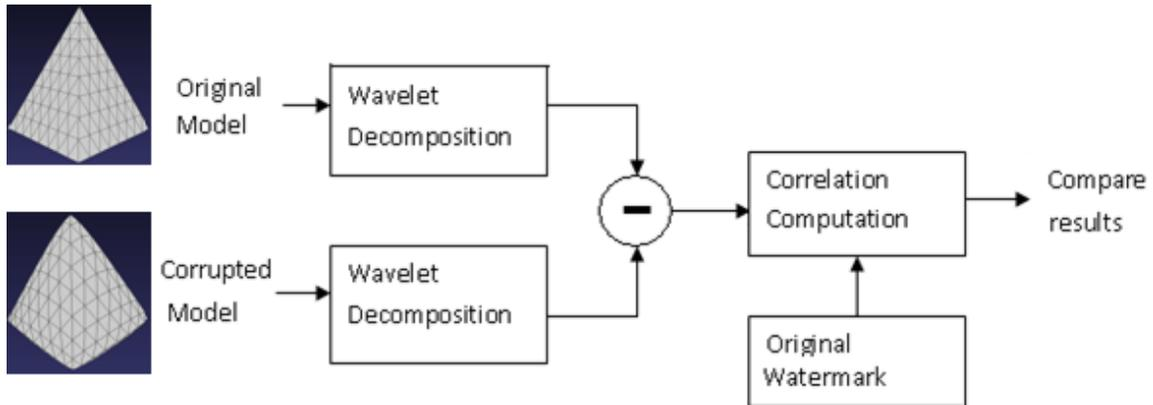
Figure 4.7: Block diagram for watermark extraction
