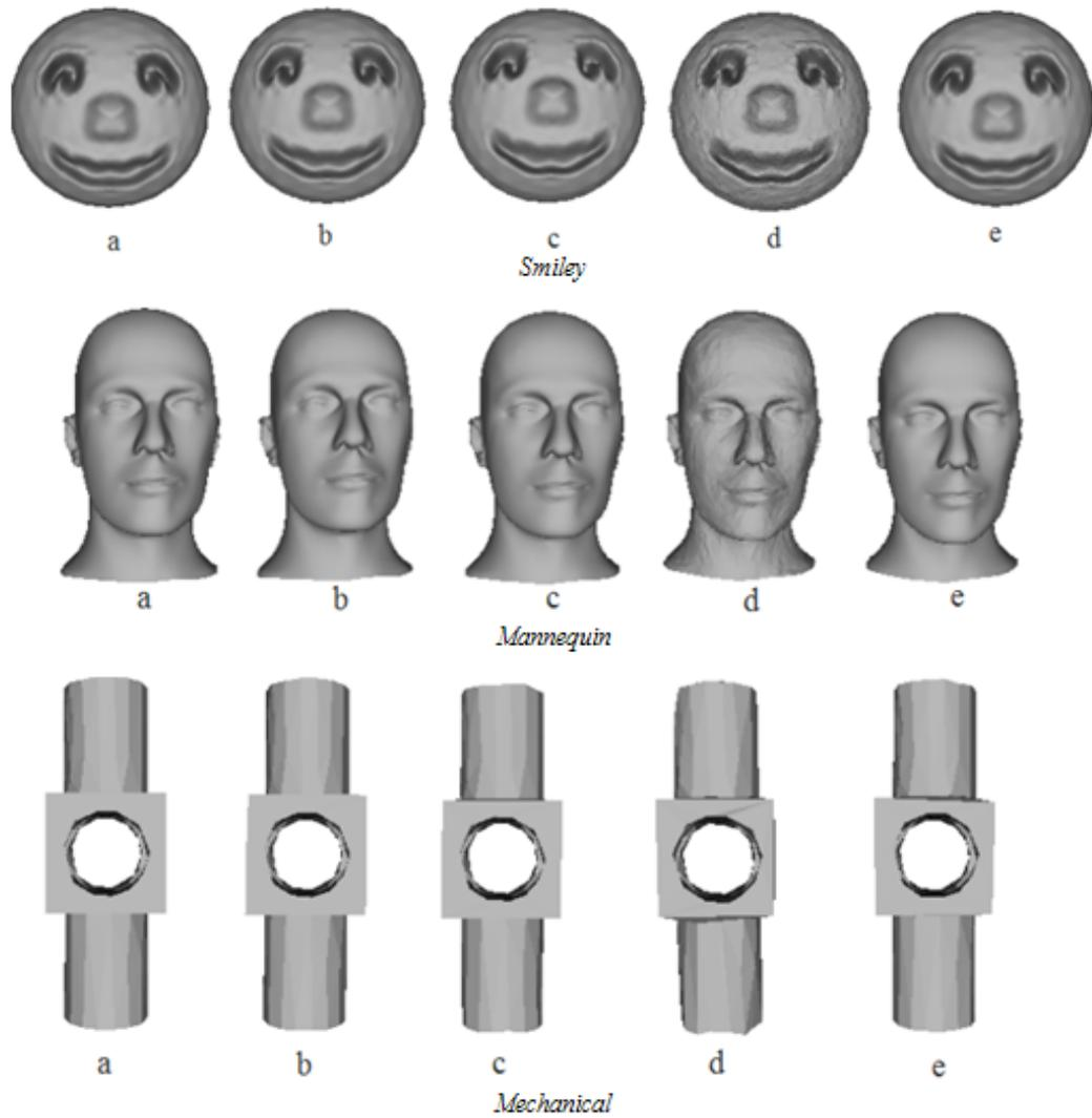
Figure 5.10: Watermarked 3D models: (a) original model, (b) watermarked model with a population size of 100, run for 100 generations, (c) watermarked model with a population size of 20, run for 100 generations, (d) watermarked model with a population size of 20, run for 20 generations, and (e) watermarked model with a population size of 100, run for 20 generations.
