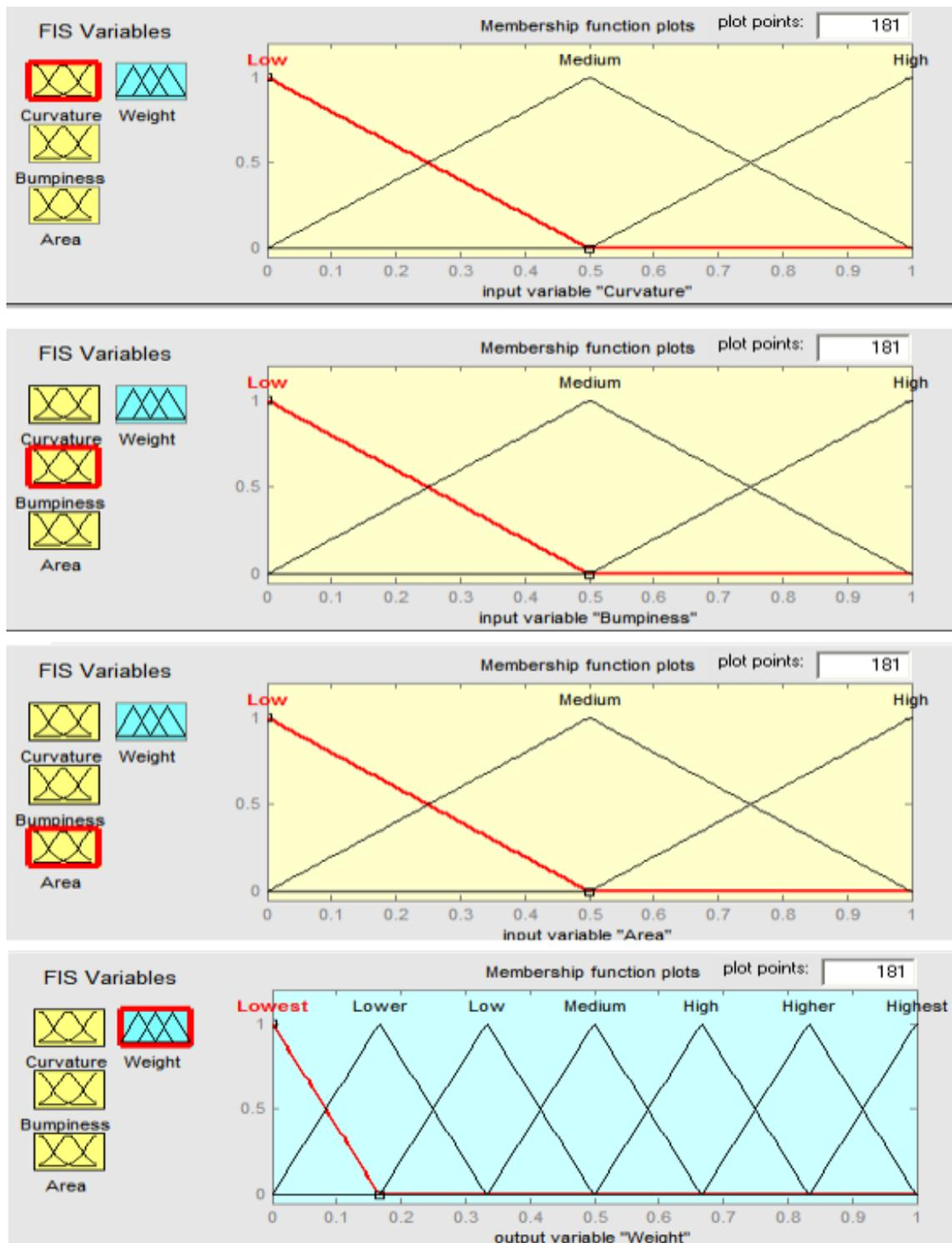
Figure 4.5: Membership functions for Fuzzy Inputs and Outputs
