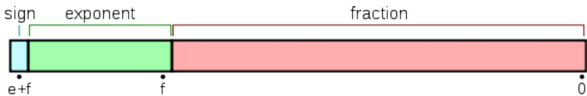
Figure 3.6: Floating Point Representation of Vertex Coordinate
