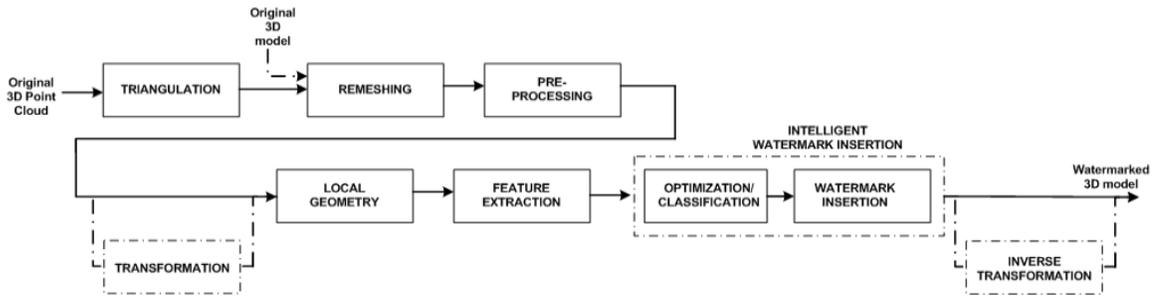
Figure 3.1: Third Generation Watermarking Block Diagram
