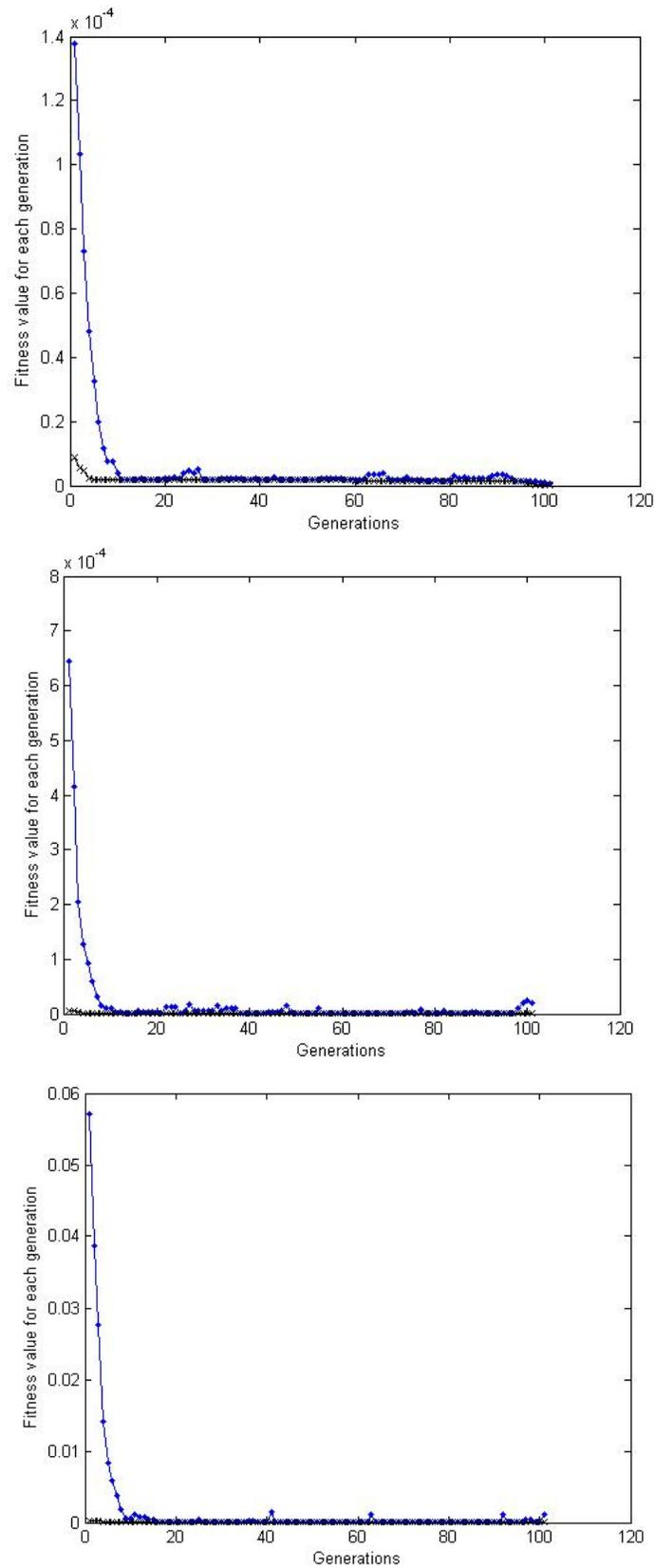
Figure 5.3: In running for 100 generations with a population size of 100, the change in best fitness value and the mean fitness value: (a) for vertex index 10 of the Smiley, (b) for vertex index 10 of the Mannequin, and (c) for vertex index 20 of the Mechanical.
