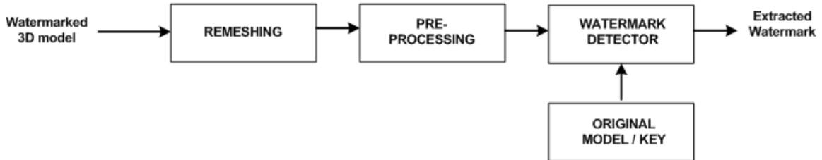
Figure 3.5: First Generation Watermarking Block Diagram
