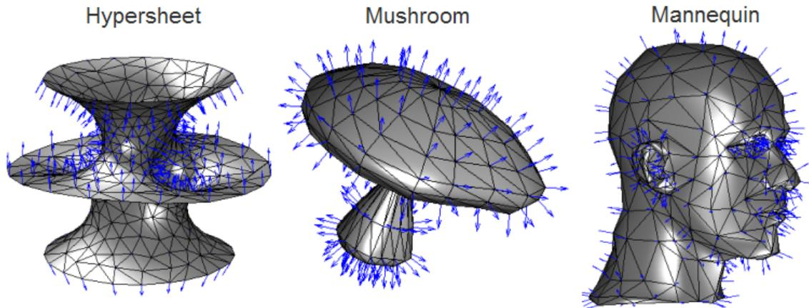
Figure 6.4: Curvature Estimation From Normal Vector Distribution
