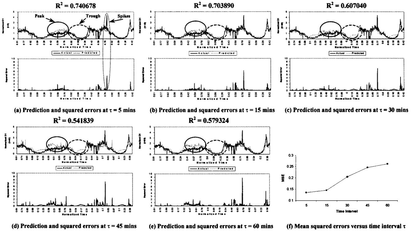
Fig. 10. Prediction of lane 1 density using GenSoFNN-CRI(S) (Training set is CV1).
