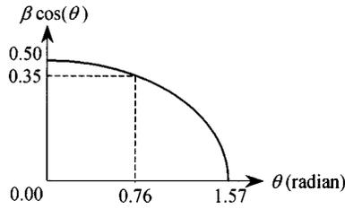
Fig. 3. Modeling of the plasticity parameter  $\beta$ .
