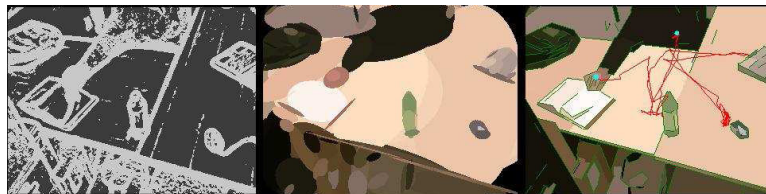
FIGURE 10.3 Left: An example of the feed-forward process. Dark-gray pixels are preserved, Light-gray pixels are re-clustered. Center: MSERs are modeled and displayed using ellipses and average colour-values. Right: An example of MSER image segmentation. Regions are filled with their average colour, detected lines are shown in green, the path of the tracked hand is represented as a red line.
