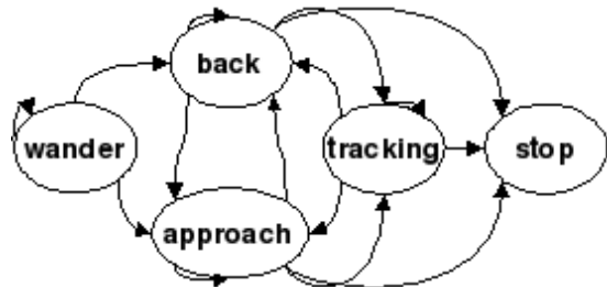
Fig. 2. HMM structure for the follow activity
