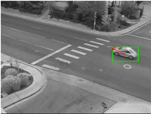
Fig. 5. An example foreground object detection (the green bounding box) and displacement vector calculated using SIFT feature matching (the red arrow).
