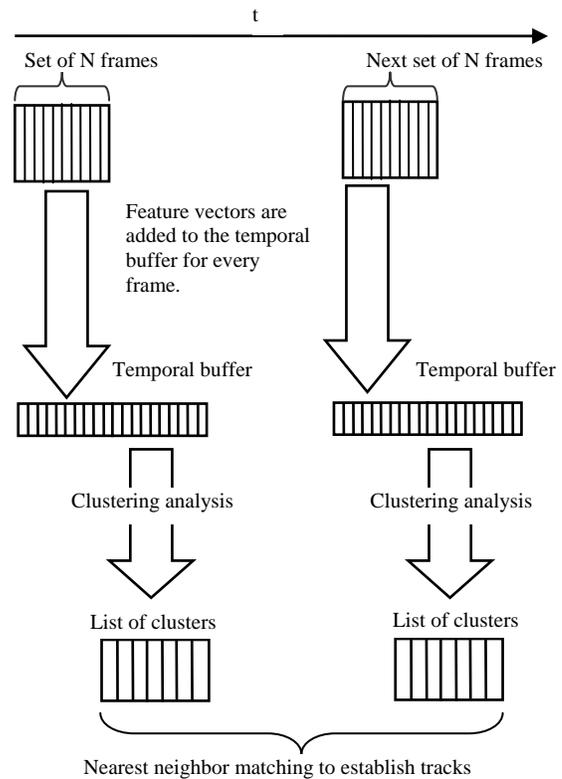
Fig. 3. Block diagram of the piecewise feature clustering.
