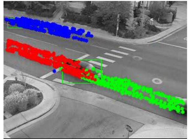
Fig. 8. An example showing three objects being tracked simultaneously. The circles of three different colors represent three different tracks.
