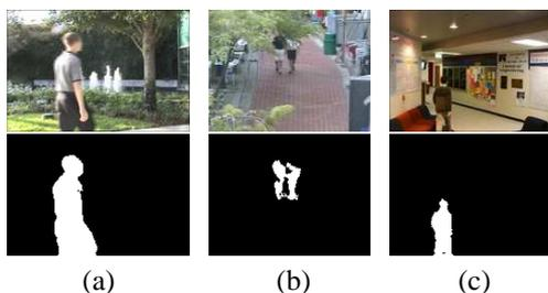
Figure 6. Results of the foreground detection using the proposed incremental SVDD to the background modeling. Top row: Original videos. Bottom row: Detection results.
