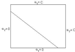
Figure 2. The two Lagrange multipliers should satisfy the inequality constraint (3) and the linear equality (7).
