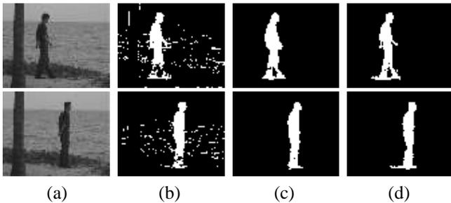
Figure 5. Water surface video: comparison of methods in presence of irregular motion. (a) Original frame, (b) MoG, (c) AKDE, (d) INCSVDD.
