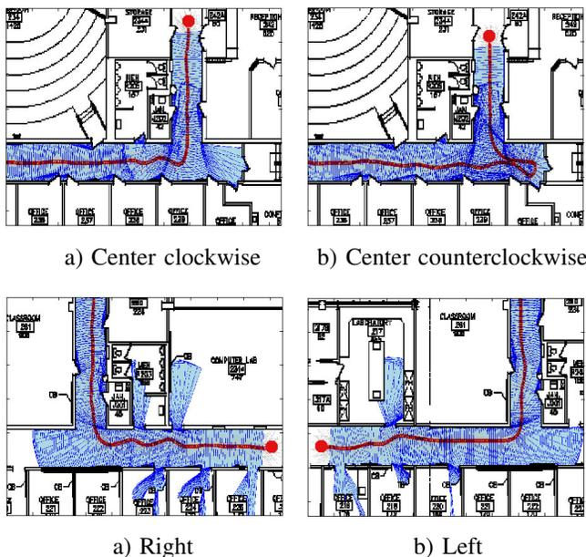
Fig. 4. Robot trajectories using controllers from the different navigation styles. The robot's path is indicated in red. The starting position is indicated by a red circle.
