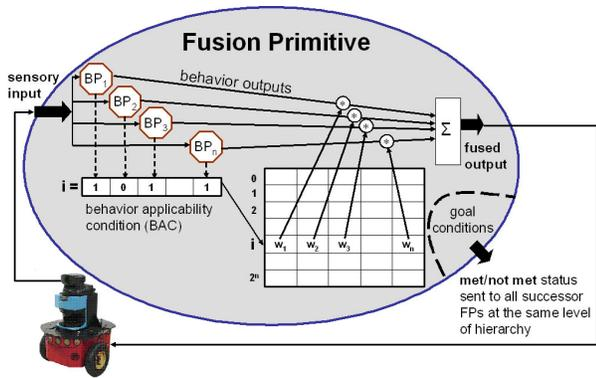
Fig. 1. Representation of a fusion primitive, the key component of the architecture. BP: behavior primitives.
