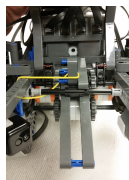
Figure 7: The ramp and extension used for pushing the ball over the wall
