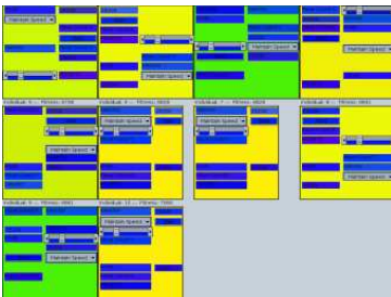
Evolved UIs at generation 200. The UIs have blue widgets, as was the assumed user preference (a subjective design criterion). Also, the UIs have high contrast between background and foreground (the result of an objective design and evaluation criterion).
