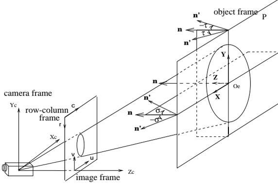
**Figure 1. Camera perspective projection model**
