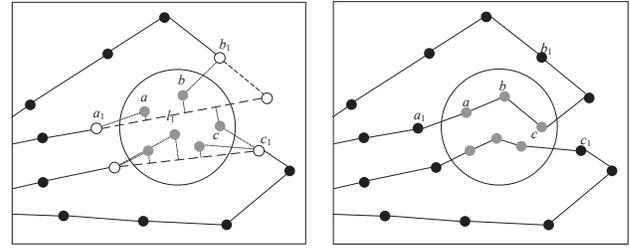
Fig. 3. Illustration of the process of inserting nodes by using the proposed insertion operator.
