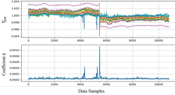
Fig. 2: Line outage detection using rank signatures, where coefficient  $\eta$  of the positive sequence voltage magnitude signal is shown.
