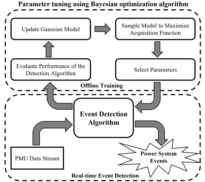
Fig. 1: The overall framework of the proposed event detection algorithm using Bayesian optimization for tuning parameters.
